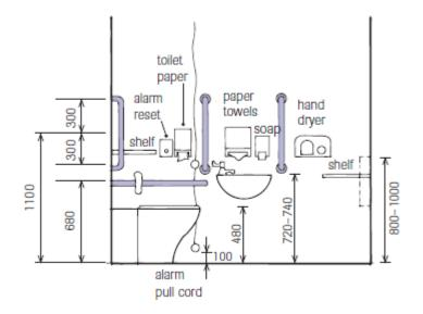
An **ambulant accessible toilet** is similar in size to a standard toilet facility or cubicle but it has a higher toilet pan, grab rails and usually an outward opening door. It will not accommodate a wheelchair and has no facilities for colostomy bag users. Key dimensions are shown below:
