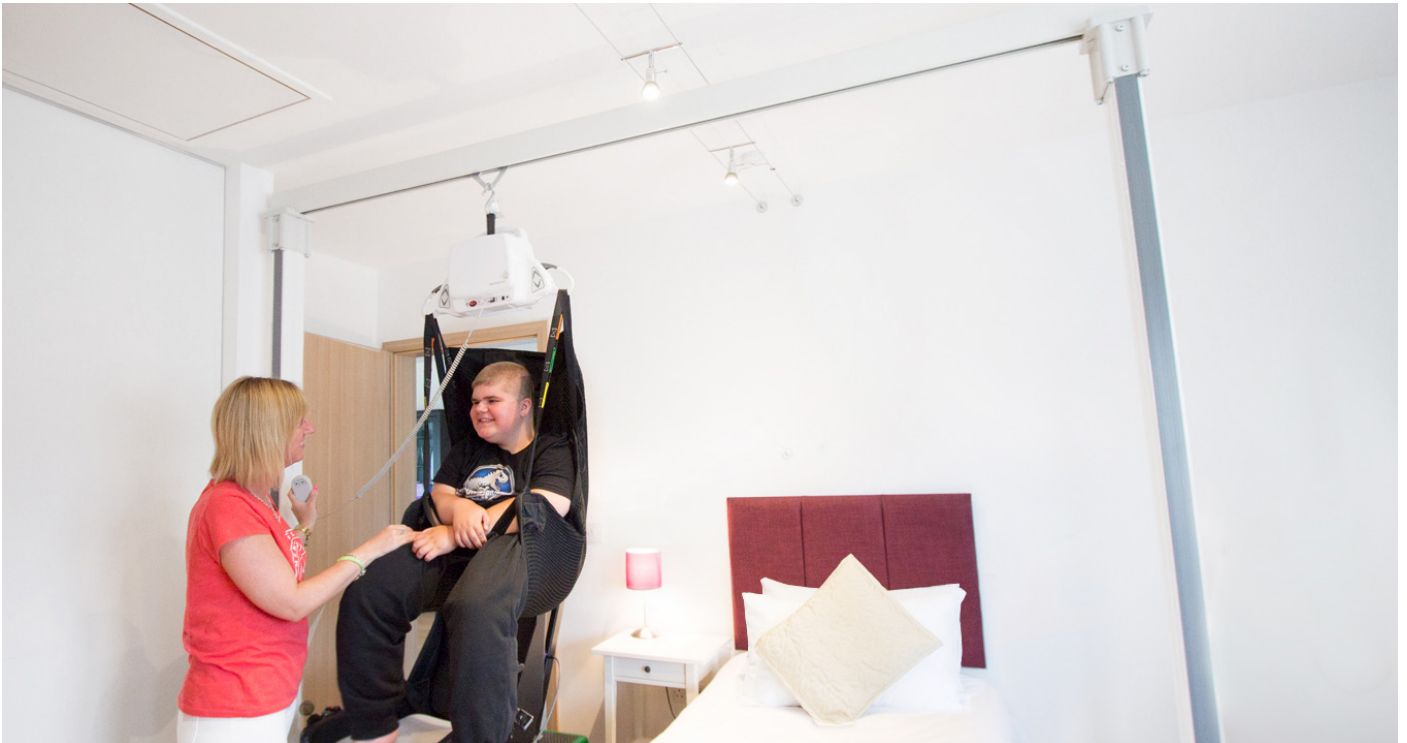
Portable hoist on a gantry system.
